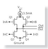
The termination is 100 ohms connected between the Out and Out\*. The InX nodes are driven from the internal circuitry. The output states are:
