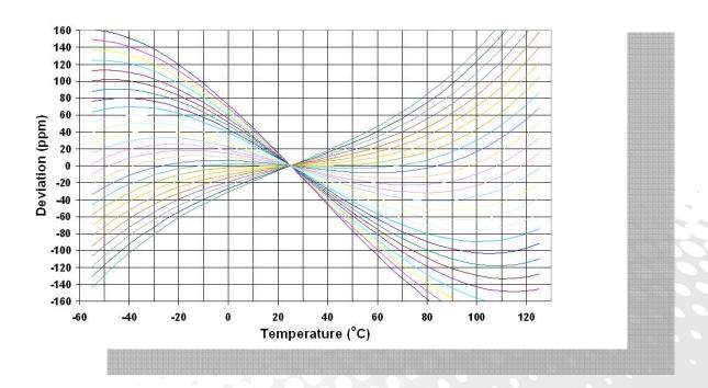
Each curve is a variation of 2 minutes of arc of the cut through the atomic planes of the quartz crystal.
