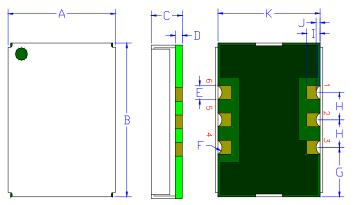
FR4 PCB Base: Solder masked All via holes tented on bottom Copper Clad ½ oz. Typical Gold plated 0.02 μinch (0.5 μm) Label:
