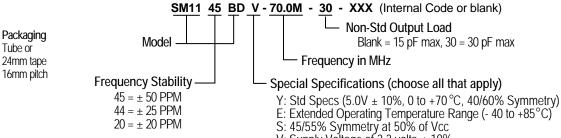
V: Supply Voltage of 3.3 volts ± 10% W: Supply Voltage of 2.5 volts ± 5%
