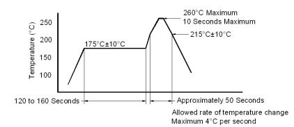
The part may be reflowed 2 times without degradation (typical for lead free processing).
