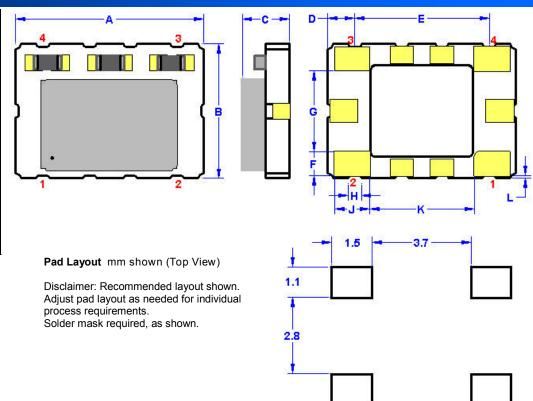
(Not to Scale) Contacts (pads): Gold 11.8 to 39.4 µinches (0.3 to 1.0 µm) over Nickel 50 to 350 µinches (1.27 to 8.89 µm)
